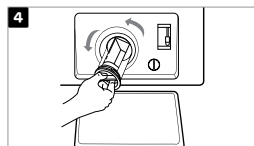
Open the pump filter by turning it counter clockwise. Clean the pump filter under running water.
